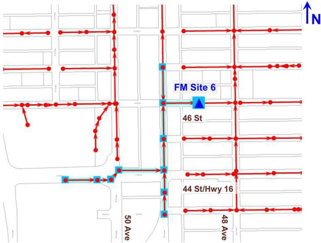
Figure 1.7: Flow Monitor Site 6 Location and Upstream Sewershed
