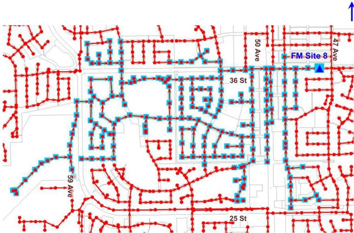
Figure 1.9: Flow Monitor Site 8 Location and Upstream Sewershed
