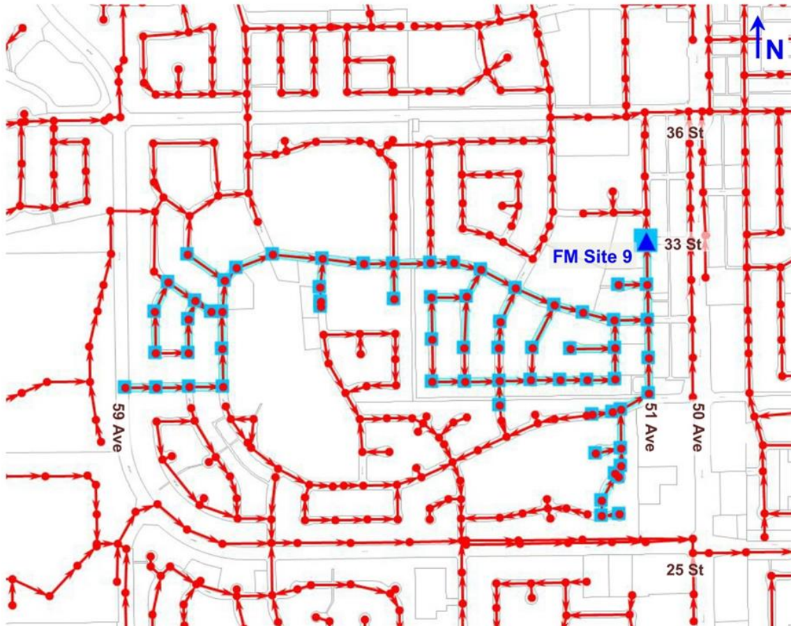
Figure 1.10: Flow Monitor Site 9 Location and Upstream Sewershed
