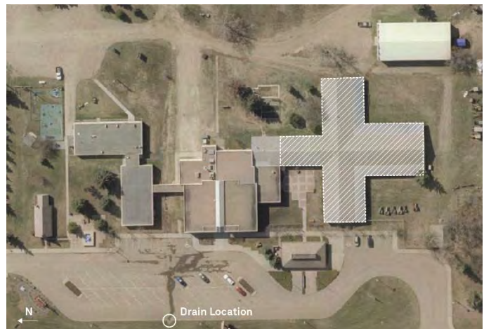
FIGURE 2 - Single Drain in Parking Lot for entire NE Site Area
